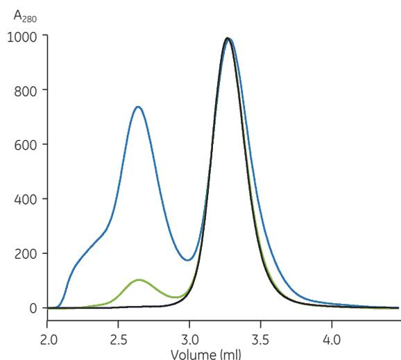
**Fig 2.** SEC analysis of the MAb in the Capto adhere step—sample before purification (green), purified fraction (black) and strip fraction (blue). The curves were normalized with respect to the monomer peak of the purified fraction.
