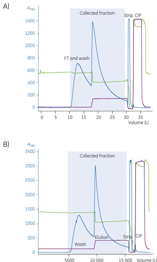
**Fig 4. A)** Chromatogram from the Capto adhere step with ReadyToProcess columns.  $A_{280}$  trace is shown in blue, pH in green and conductivity in lilac; **B)** Chromatogram from the Capto adhere step with AxiChrom columns.  $A_{280}$  trace is shown in blue, pH in green, and conductivity in lilac. The difference in absorbance is due to the difference in path length between the two systems.
