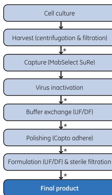
**Fig 1.** Flow scheme of the purification process. In-process filtration of the sample to reduce bioburden is indicated with asterisks.
