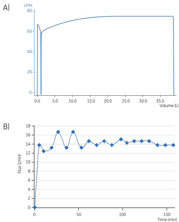
**Fig 5.** Flux curves from the buffer exchange step. **A)** traditional format with Kvick Lab cassettes; **B)** with ReadyToProcess.
