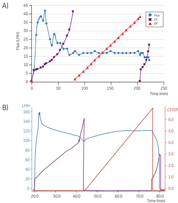
**Fig 6.** Flux curves from the formulation step. Flux is denoted by blue, concentration factor (CF) by lilac, and diafiltration factor (DF) by red. **A)** traditional format with Kwick Lab cassettes; **B)** with ReadyToProcess.
