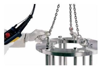
3 Carefully lift the the column just off the floor and then lower it again. This will position the center the column aligned with the hoist.
