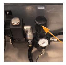
4 Connect the panel of pneumatic nozzle control hoses to the connection panel on column.
