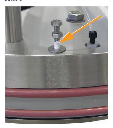
4 Screw down the nut on each of the bed support retaining screws.
