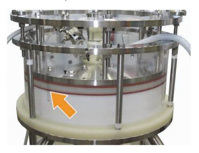
If the column has a stainless steel bed support then stop the pump when the packed bed reaches 0.5 cm from the top bed support, or when a defined compression factor is reached.
