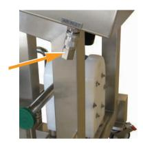
Make sure that the pressure regulator for the compressed air located inside the cabinet is set to the correct bar g pressure for your operation. Adjustments are made by turning the knob that is indicated below.
