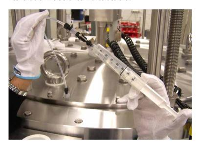
3 Close the flushing port valve.
