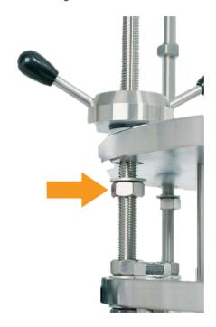
2 Make sure that the nuts are at the same distance from the flange. Use a caliper or steel rule.
