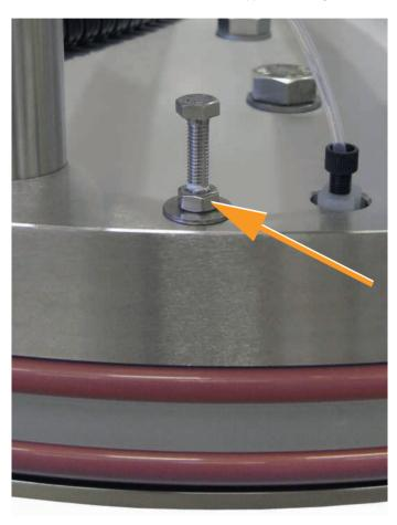
Hold the top of the bed support retaining screw in place with a ring spanner or socket spanner, and then slowly tighten the nut on each of the screws using a calibrated open torque wrench, as shown in the illustration.
