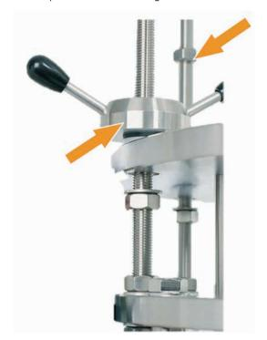
2 Make sure that the nuts are at the same distance from the flange. Use a caliper or steel rule.
