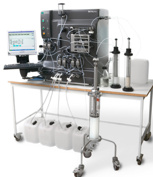
Fig 5. Scale-up of PlasmidSelect Xtra process with pilot-scale columns connected to an ÄKTApilot™ system.
