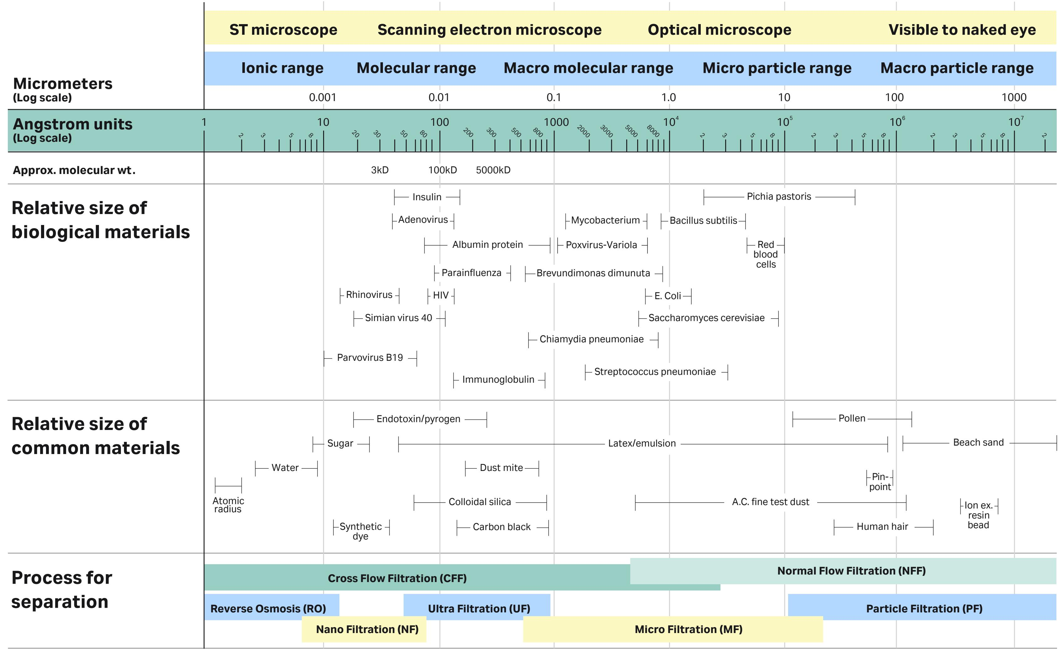
Note: 1 micron ( $1 \times 10^{-6}$  meters)  $\approx 4 \times 10^{-5}$  inches (0.00004 inches); 1 angstrom unit =  $10^{-10}$  meters =  $10^{-4}$  micrometers (microns)
