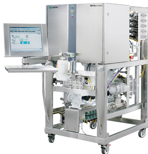
Fig 1. A standard, gradient ÄKTAprocess™ system has the ability to perform the first level of inline conditioning.
