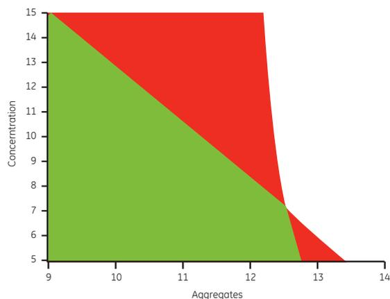
**Fig 6.** Sweet spot plot of the polishing step with a criteria of yield > 85%; monomer purity > 99% (equivalent to an aggregate content of < 1%). The region within which all the criteria were met is represented in green, red represents a region in which only two of the criteria were met and white represents a region in which only one criterion was met. The other criteria were a load of 60 g/L, an elution pH of 6.1, and an elution NaCl concentration of 300 mM.
