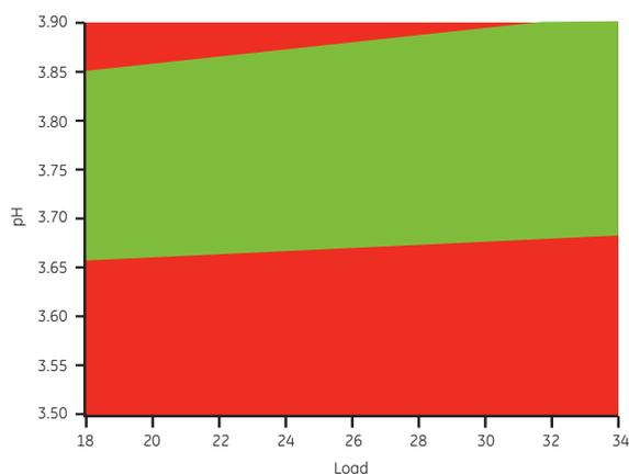
**Fig 2.** Sweet spot plot of the capture step with the following predefined criteria: yield > 90%, aggregate content < 15%, and HCP content < 70 ppm. Green = all criteria met, red = two criteria met. Load is expressed in g/L.
