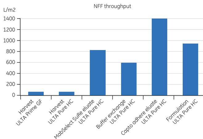
**Fig 12.** Membrane throughput expressed as volumetric load per membrane area for a filtration step in 30 min. The harvest process produced low membrane capacity because of high particle and impurity levels. The subsequent filtrations steps were limited by product concentration rather than impurities.
