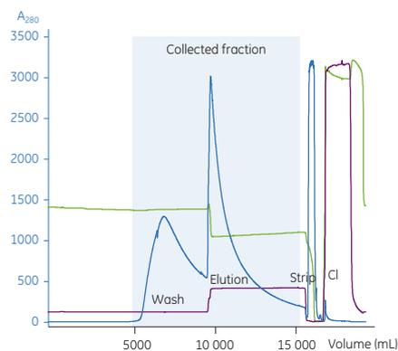
**Fig 9.** Chromatogram from the Cpto adhere step (2<sup>nd</sup> cycle).  $A_{280}$  trace is shown in blue, pH in green, and conductivity in brown.
