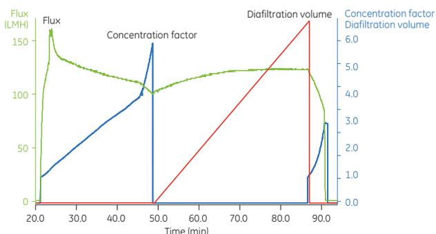
**Fig 11.** Schematic representation of process performance (during formulation) showing the changes in flux vis-à-vis the concentration factor (CF) and diafiltration volume. The Capto adhere eluate was concentrated 6-fold, diafiltered 7 times, and then concentrated a further 3-fold.
