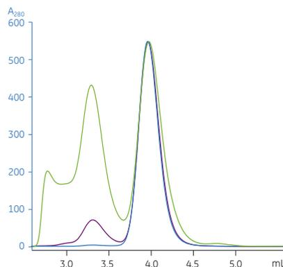
**Fig 10.** SEC analysis of the monoclonal antibody sample in the Cpto adhere step: sample before purification (purple), purified fraction (blue) and strip fraction (green). The curves were normalized with respect to the monomer peak of the purified fraction.
