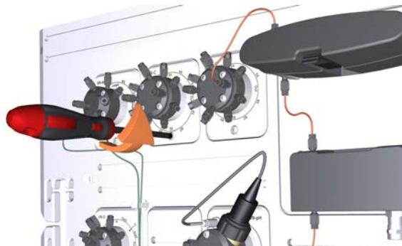
3 Remove the valve module.
