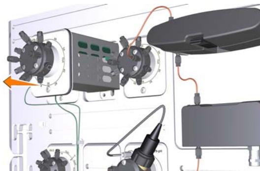
4 Disconnect the cable and secure it in the slit.
