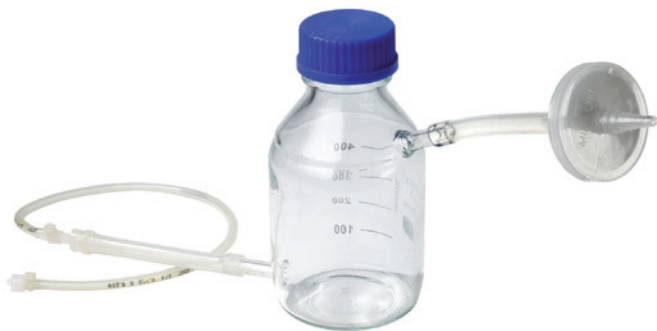
Fig 1. (A) WAVE Bioreactor 2/10 system with Perfusion Controller. (B) Custom-made transfer flask; glass bottle with two spouts; one is coupled to a sterile filter and the other to transfer tubing.
