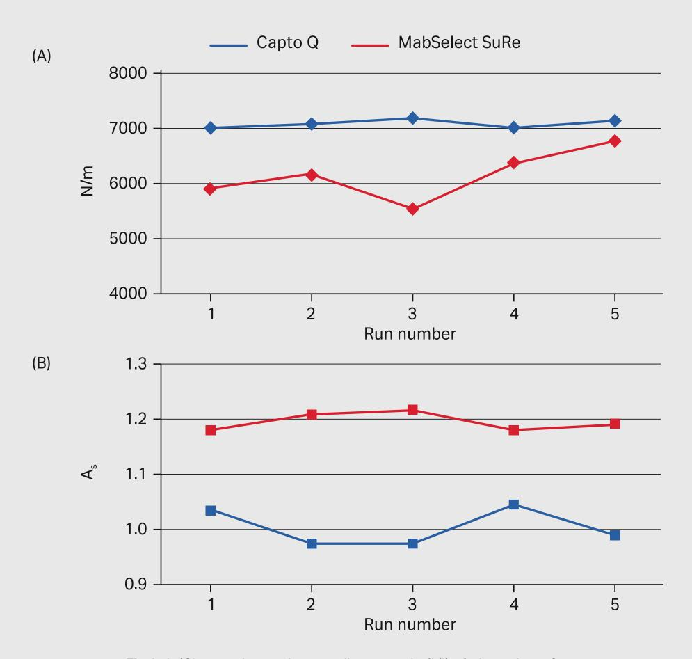
**Fig 2**. AxiChrom columns show excellent reproducibility independent of operator or column size. Repeated packings, by two to three different operators, of Capto Q in AxiChrom 50 at 40 cm bed height and MabSelect SuRe packed in AxiChrom 1600 at 20 cm bed height. The degree of variation in plates per meter (N/m) and asymmetries ( $A_s$ ) is similar in AxiChrom 50 and 1600 columns, demonstrating both reproducibility and scalability.
