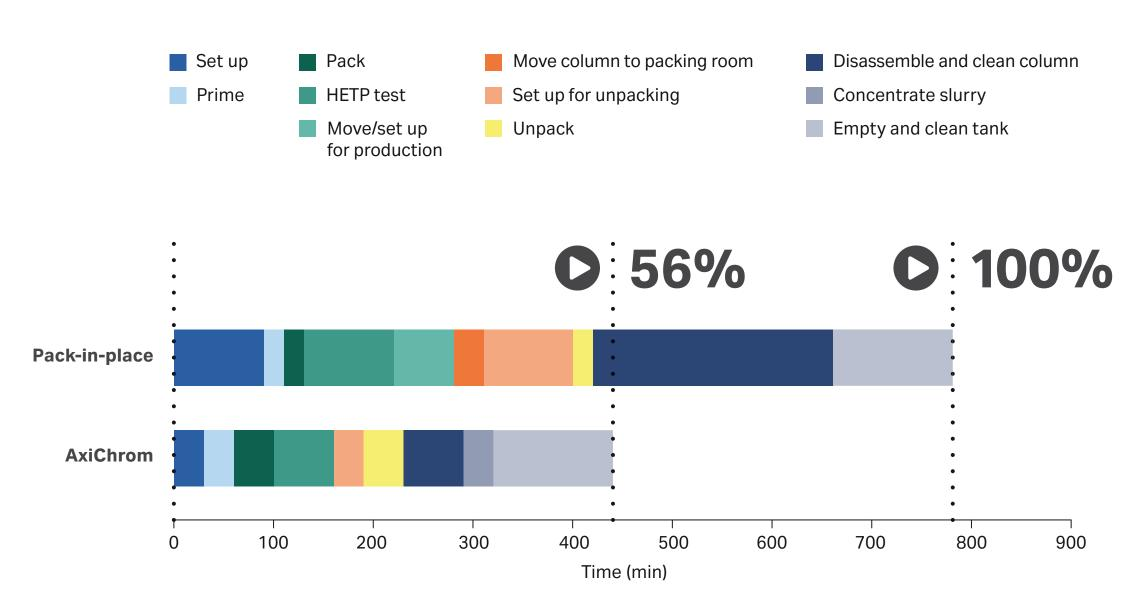
**Fig 1.** Packing, unpacking, and maintenance of an AxiChrom column only takes 56% of the time required for a traditional column. Successful packing at first go ensures that labor, resin, and water costs are reduced. An optimally packed, stable bed together with straightforward handling and maintenance will also give secured uptime in operation. Data from Cytiva assessment studies.
