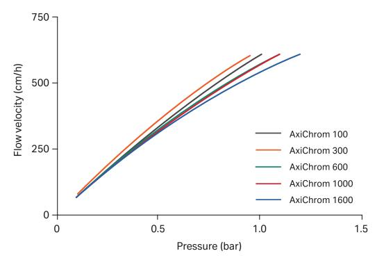
**Fig 5.** Regression curves of pressure-flow tests for MabSelect SuRe in 20°C water at 20 cm packed bed height in AxiChrom 100, 300, 600, 1000, and 1600 equipped with stainless steel bed supports. Pressure/flow curves provide a simple, yet effective illustration of column and resin performance in terms of the maximum velocity at which the process can be run. MabSelect SuRe can be run at 500 cm/h with a back pressure of less than 2.0 bar. System/ tubing pressure is excluded.
