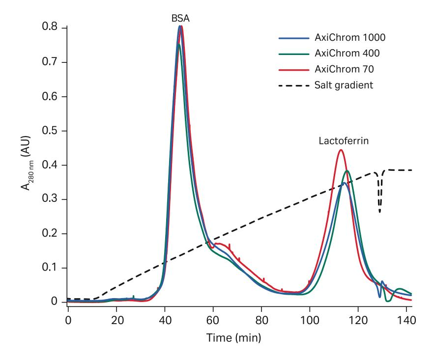
**Fig 3.** Separation of bovine serum albumin (BSA) and Lactoferrin on SP Sepharose Fast Flow in different AxiChrom columns demonstrates real scalability within the AxiChrom platform.
