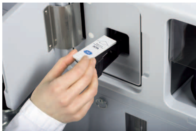
Fig 1. Sensor Chip NTA is used for the study of molecular interactions between histidine-tagged proteins immobilized on the chip and numerous analytes.
