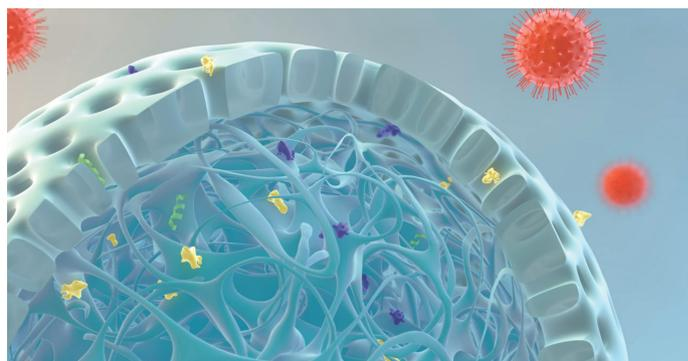
**Fig 1.** Schematic representation of the principle for core bead technology, showing a bead with the inactive shell, pores in the shell, and the ligand-activated core. Small proteins and impurities (colored green, yellow, and purple) penetrate the core, while target viruses (red) and larger proteins are excluded from the resin and are collected in the flowthrough.
