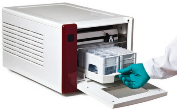
Fig 10. Fraction collector F9-C holds cassettes for a variety of tubes from 3 to 50 mL as well as 24-, 48-, and 96-deep-well plates.
