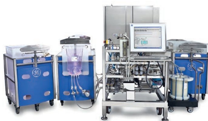
Fig 1. ReadyToProcess column connected to a BioProcess IC system. Buffer and sample management was achieved by a combination of ready-to-use liquid-handling components such as ReadyCircuit bags and tubing, ReadyMate™ Disposable Aseptic Connectors (DAC), and ReadyKart mobile processing stations.
