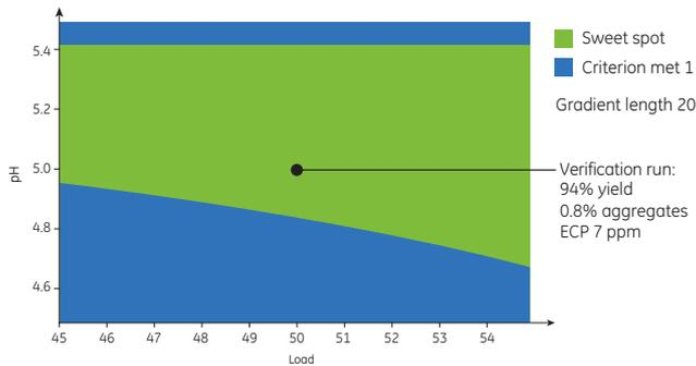
**Fig 6.** The sweet spot plot, for a gradient length of 20 column volumes, showed a wide experimental space where both the criteria of high yield (> 90%) and maximum aggregate content of 1% were met. A verification run was performed within the sweet spot to further validate the model. When using a load of 50 mg/mL and a pH of 5, the monomer yield was 94%, with 0.8% aggregates and an ECP level of 7 ppm.
