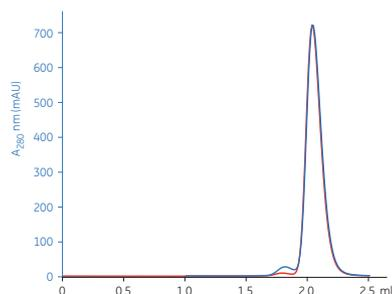
Fig 9. Normalized chromatogram from the SEC analysis of the Capto L elution pool (blue trace) and final product (red trace).
