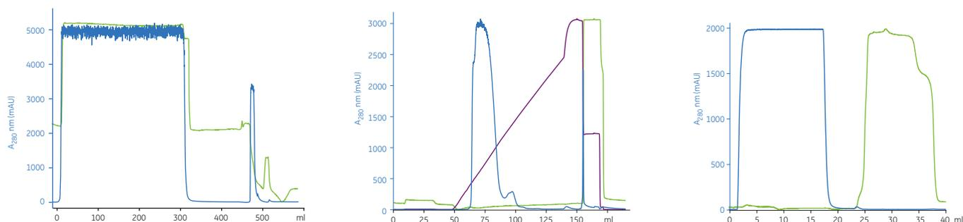
Fig 8. Chromatogram from the verification runs in the three-step process. Traces are UV (blue), conductivity (purple), and pH (green).
