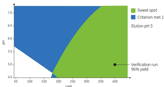
**Fig 4.** Sweet spot analysis for yield and ECP content using Capto L in the capture step. Criteria were an ECP content of 2-30 ppm and a yield of 95%-100%. The green surface shows conditions where both criteria were met. A verification run was performed within the sweet spot and results were: 96% Fab yield containing only 12 ppm of ECP.
