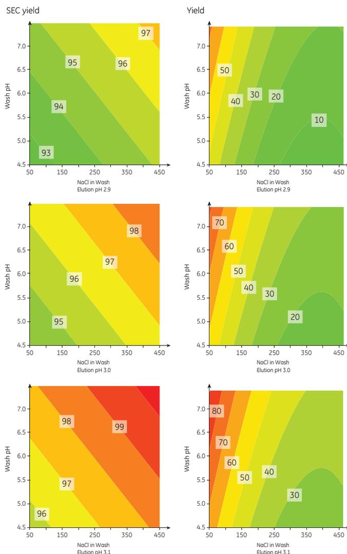
**Fig 3.** Contour plots at three different elution pH values, showing the responses for yield determined by size exclusion chromatography (SEC) and ECP. Optima for yield and ECP did not coincide. The SEC yield is highest in the upper right corner (high salt content in the wash and high wash pH) while the lowest values for ECP were obtained in the lower right corner (high salt content in the wash and low wash pH).
