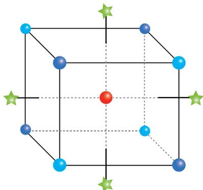
**Fig 2.** For all three steps, the optimization study used a Central Composite Circumscribed (CCC) design. This high resolution design supports quadratic interactions, while the star distance points eliminate confounding between interactions and quadratic terms.
