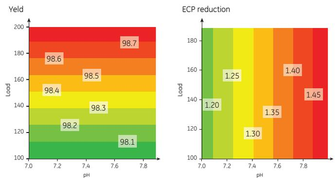
**Fig 7.** Contour plots for yield (left) and ECP reduction (right) using Capto Q. The only factor significantly affecting yield was the load - the higher the load the higher the yield. The DoE showed that the ECP-reduction factor was independent of load and residence time. The only significant factor was the pH: the higher the pH the better the ECP reduction.
