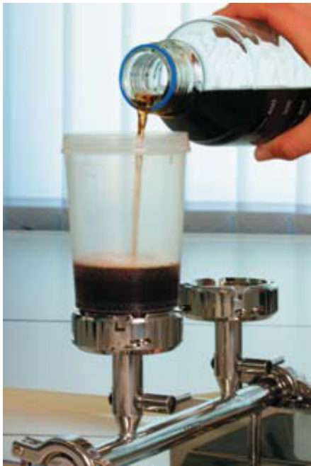
Fig 3. Liquid is poured into funnel and vacuum is activated.
