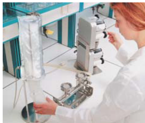
Fig 1. By taking a new pre-sterilized funnel, a membrane is dispensed automatically. (Workflow continued on next page).
