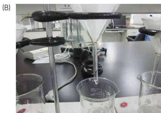
Fig 4 A and B. Second filtration step using Grade 42 filter paper.
