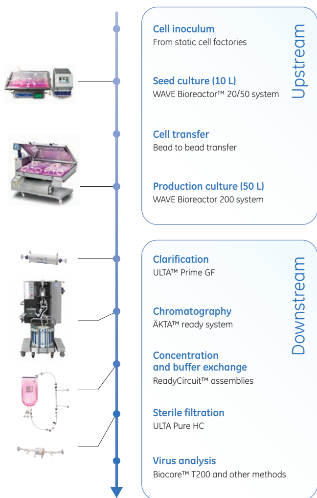
Fig 2. Overview of the production process of whole live influenza virus using ReadyToProcess equipment.
