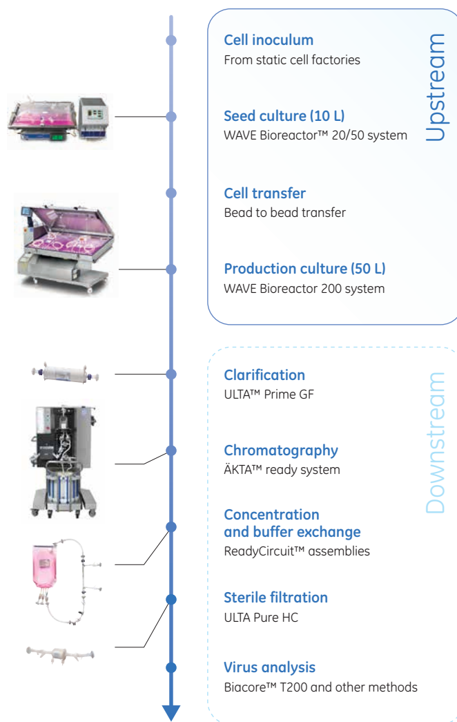
Fig 1. Overview of the production process of whole, live influenza virus using ReadyToProcess equipment.
