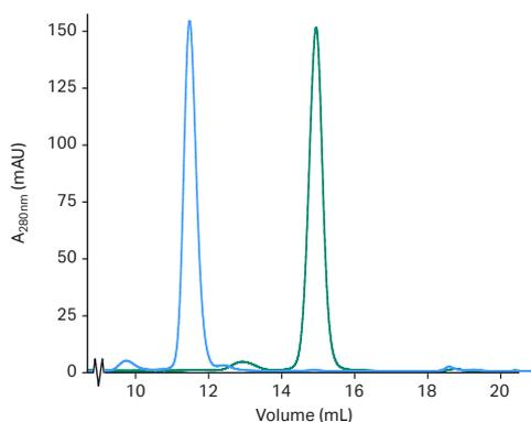
**Fig 9.** Overlay of two chromatograms for analysis of a papain-digested IgG antibody using Superdex 200 Increase 10/300 GL. Blue chromatogram corresponds to intact mAb and green chromatogram to Fab fragment.
