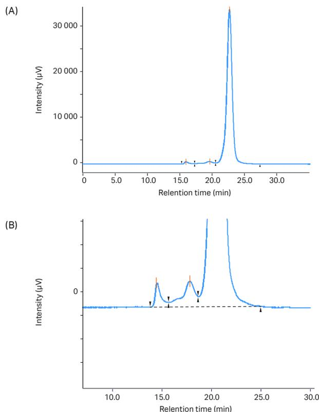
**Fig 8.** Analysis of monoclonal mouse IgG<sub>1</sub> antibody aggregates using Superdex 200 Increase 10/300 GL. (A) Chromatogram without magnification. (B) Magnified chromatogram showing details of aggregates, dimer, and monomer peaks.
