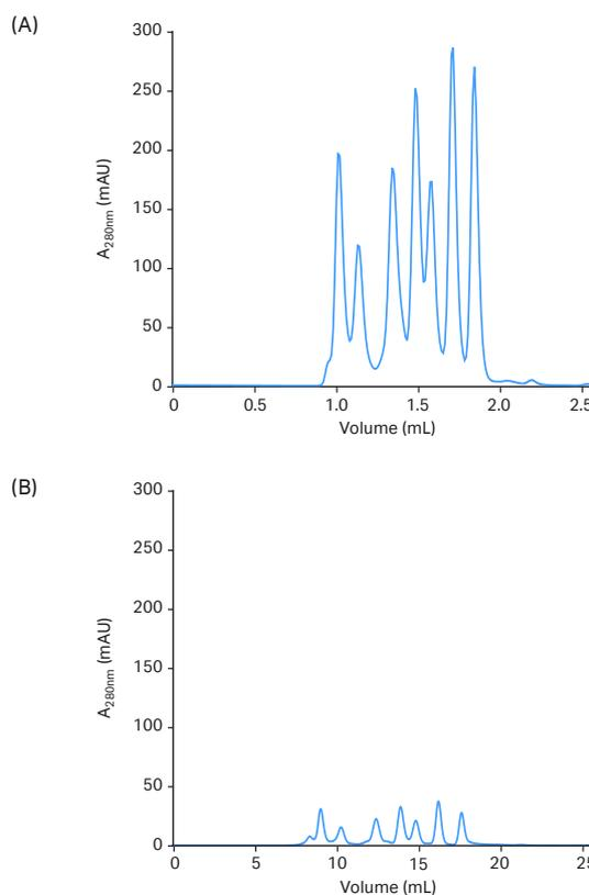
**Fig 4.** A small volume (20  $\mu$ L with a total of 370  $\mu$ g protein) of a sample mixture containing seven proteins was separated on (A) Superdex 200 Increase 3.2/300 column and (B) Superdex 200 Increase 10/300 GL column. Both graphs show the same scale for UV detection.
