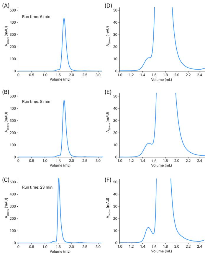
**Fig 5.** Effect of flow rate on cycle time and resolution of mAb monomers and dimers using Superdex 200 Increase 5/150 GL. (A) Run at a flow rate of 0.6 mL/min, resulting in a 6 min separation time. (B) Run at recommended flow rate 0.45 mL/min, resulting in an 8 min separation time. (C) Run at 0.15 mL/min, resulting in a 23 min separation time. D, E, and F are amplifications of A, B, and C chromatograms. For detection, absorbance was measured at 280 nm.
