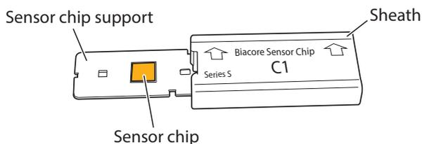
The sensor chip is fixed to a polystyrene support sheath. Each cassette, consisting of a sensor chip and sheath assembly, is individually packed under a nitrogen atmosphere in a sealed pouch.
