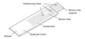
The sensor chip is fixed to a polystyrene sensor chip support. Each cassette, consisting of a sensor chip and sheath assembly, is individually packed under a nitrogen atmosphere in a sealed pouch.
