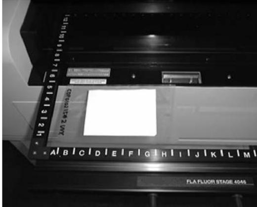
**Note:** *To reduce the effect of vibrations, place a membrane weight on top of the samples.*
