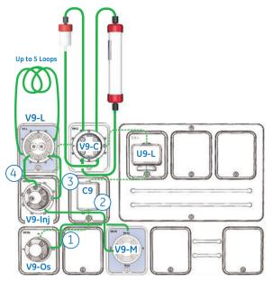
The illustration shows the two additional modules (blue) and the needed connections (green) installed on ÄKTA pure allowing two-step purification via re-injection (System pump configuration). Standard flow path shown with dash lines.
