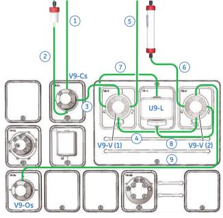
The illustration shows the flow path allowing tandem two-step purification using the UV monitor  ${\bf U9-L}$  installed on ÄKTA pure  ${}^1$ .
