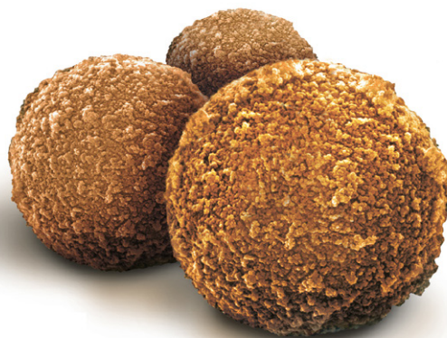
Fig 1. SEM image showing the cauliflower-like surface of the Sera-Mag™ SpeedBeads that dramatically increases the overall surface area available for binding.
