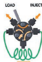
Fig 5. Image showing Manual injection valve in LOAD position and sample loop attached to ports 2 and 5.
