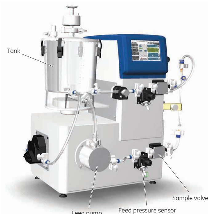
Fig 2. General location of the predetermined sampling sites on ÄKTA flux 6.
