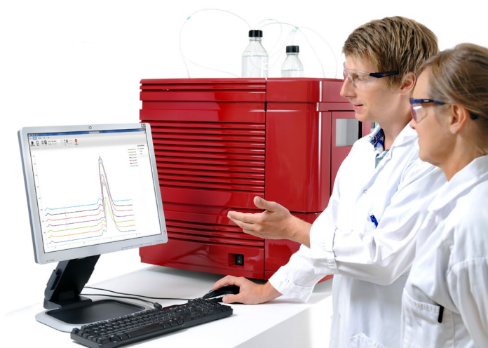
Fig 1. Evaluation of several chromatography runs using overlay view in UNICORN™ 7 control software.
