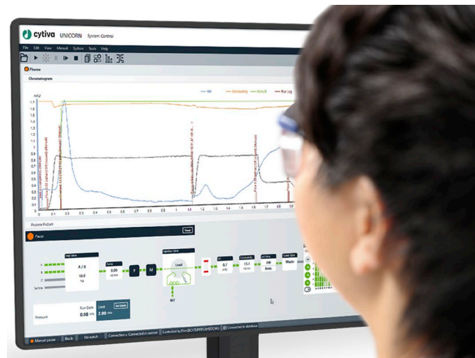
Fig 3. In System Control , the view and layout of the docking panes can be customized by dragging-and-dropping each pane.
