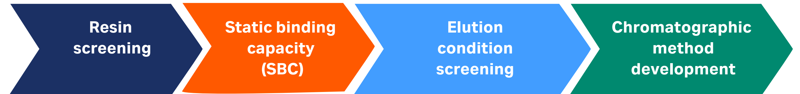
Fig 1. The Fast Trak standardized workflow applied for evaluating and selecting resins for a polishing step of a biosimilar molecule. The first part consists of screening of a wide area of conditions in a format that allows increased throughput and provides process understanding. The final part involves development of a chromatographic method to identify running conditions in an “easy-to-scale-up” approach.
