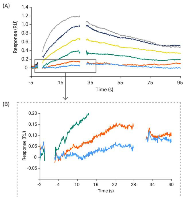
**Fig 4.** The high sensitivity of Biacore™ S200 enables confident analysis of data even in the sub-resonance units (mRU) response range. This means low density surfaces can also be used for targets with limited activity. (A) Sensorgram from a kinetic experiment between thrombin and melagatran. (B) Zoom-in on the lower concentrations demonstrating the possibility to separate curves at sub-resonance response levels.
