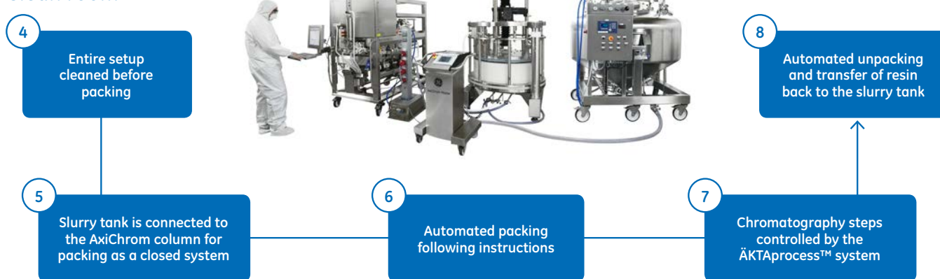
Fig 3. Contamination risks can be kept to a minimum by decreasing any manual handling of chromatography resin and buffers. This can be achieved by connecting the column, slurry tank and chromatography system in a closed system (blue boxes).
