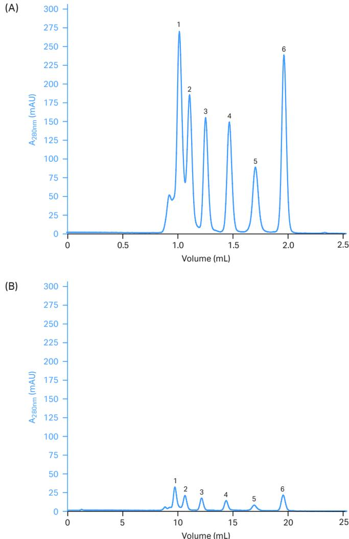
**Fig 7.** A small volume (10  $\mu$ L with a total of 110  $\mu$ g protein) of a sample mixture containing six components was separated on (A) Superdex 75 Increase 3.2/300 and (B) Superdex 75 Increase 10/300 GL. Both chromatograms show the same scale for UV detection.
