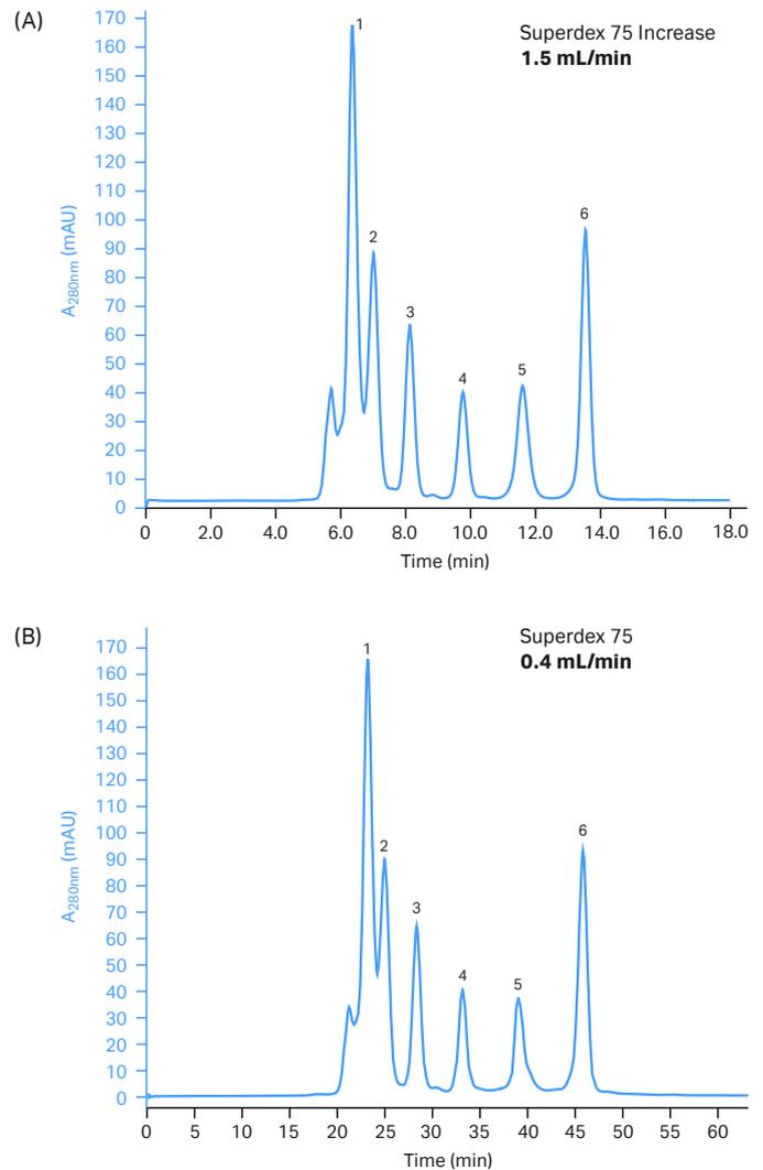
**Fig 5.** Chromatograms showing high-resolution SEC of a mixture of six standard components on (A) Superdex 75 Increase 10/300 GL at 1.5 mL/min and (B) Superdex 75 10/300 GL at 0.4 mL/min. Note that approximately the same resolution was achieved with a 3 to 4 times faster separation using Superdex 75 Increase 10/300 GL.
