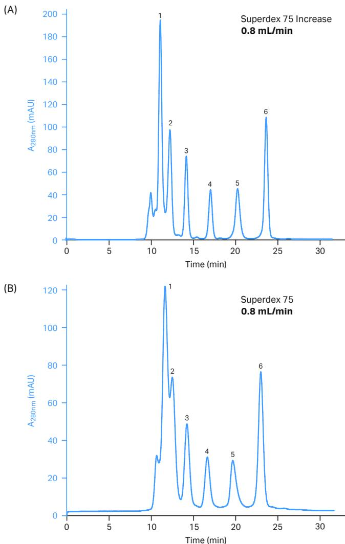
**Fig 4.** Chromatograms showing high-resolution SEC at 0.8 mL/min of a mixture of six standard components on (A) Superdex 75 Increase 10/300 GL and (B) Superdex 75 10/300 GL. Note that increased resolution gives higher peaks, with higher concentrations. In the comparison here shown, the resolution improvement with the new generation column was 40% to 120%, with the largest improvement for the higher-molecular weight proteins.
