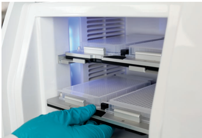
Fig 7. Biacore™ 8K accommodates up to four 96- and 384-well microplates simultaneously, all in a temperature-controlled environment for optimal assay performance or to ensure sample integrity in extended runs.
