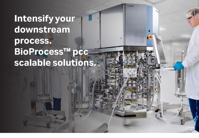
BioProcess™ pcc chromatography systems are developed for purification of your target protein in a continuous process using periodic counter-current chromatography (PCC). Continuous chromatography supports process intensification by reducing footprint and improving productivity. In addition, continuous chromatography is especially suited for purification of unstable molecules, as the short process time helps ensure stability of your target.
