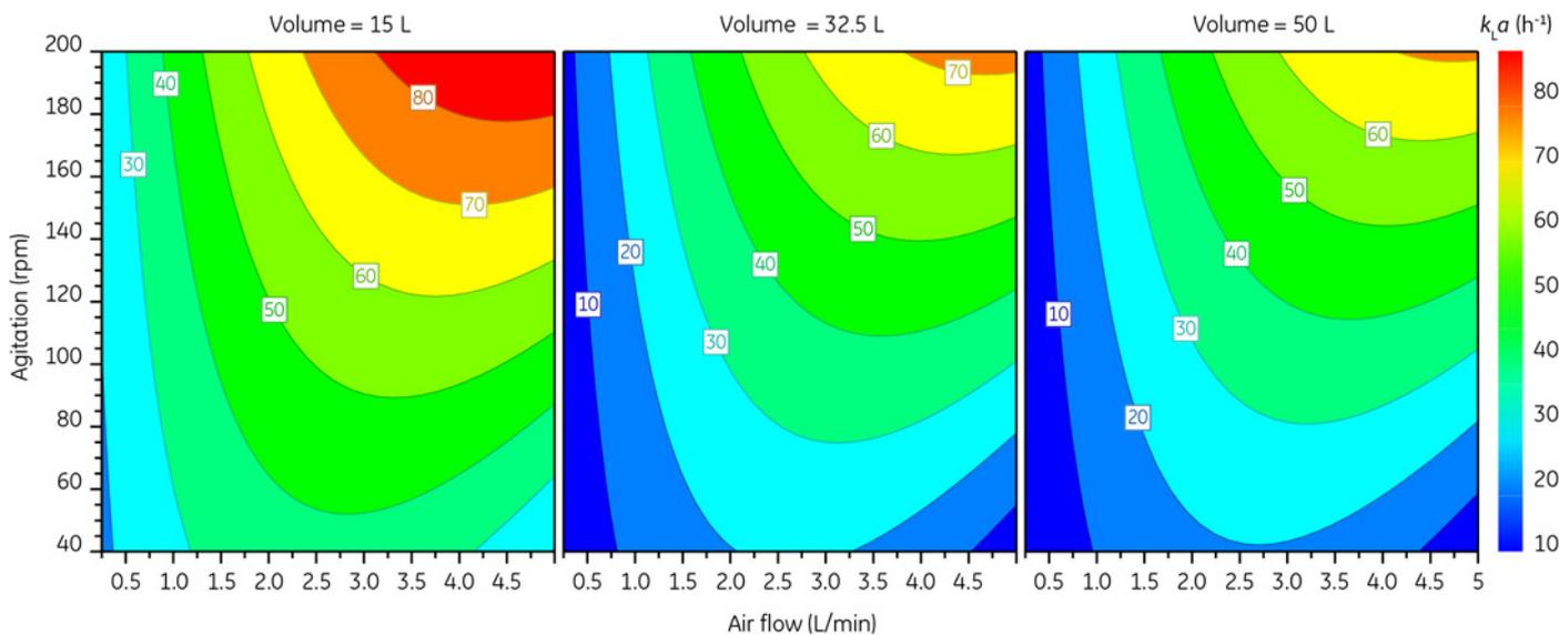
**Fig 11.** 4D response contour plot displaying  $k_L a$  obtained with the 2  $\mu\text{m}$  sparger pore size at varying air flow, volume, and agitation. The model fit ( $R^2$ ) is 0.95, the model predictability ( $Q^2$ ) is 0.88, and the residual standard deviation (RSD) of the model is  $6.37 \text{ h}^{-1}$ .
