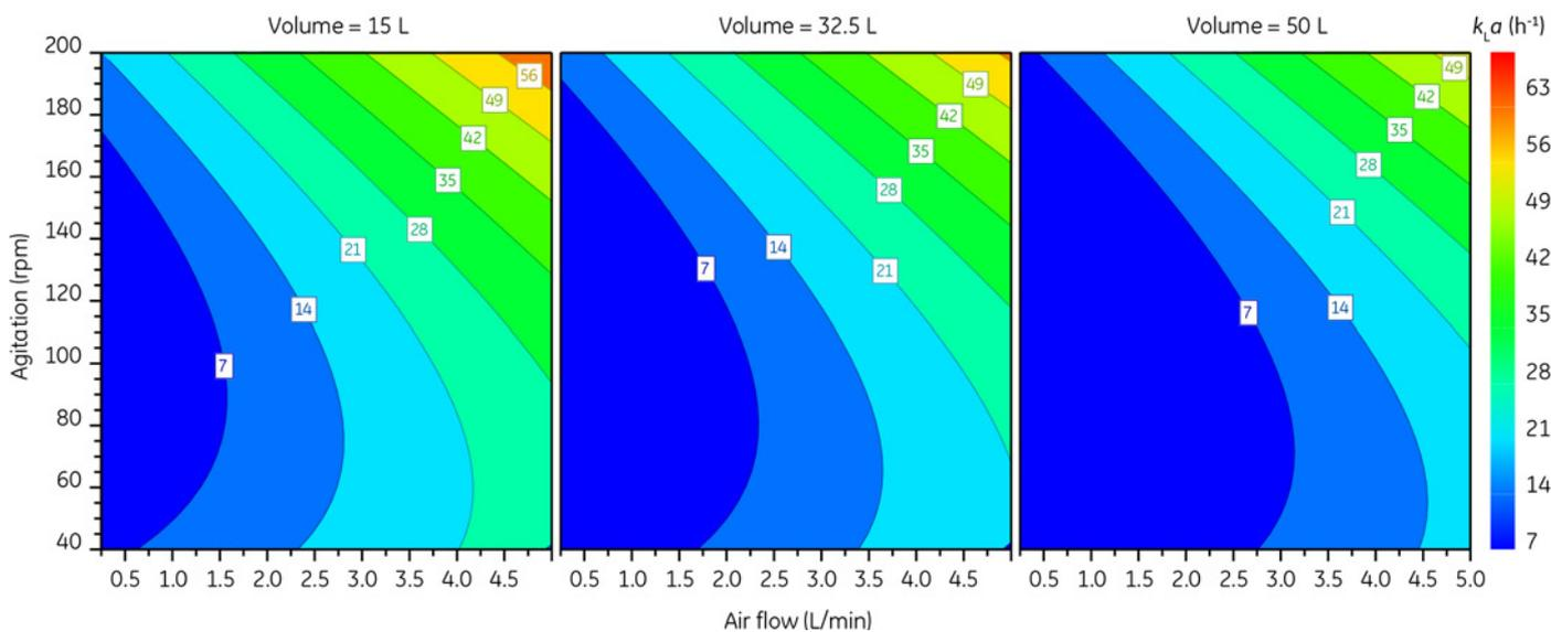
**Fig 13.** 4D response contour plot displaying  $k_L a$  obtained with the 0.5 mm sparger pore size at varying air flow, volume, and agitation. The model fit ( $R^2$ ) is 0.93, the model predictability ( $Q^2$ ) is 0.87, and the residual standard deviation (RSD) of the model is  $5.08 \text{ h}^{-1}$ .
