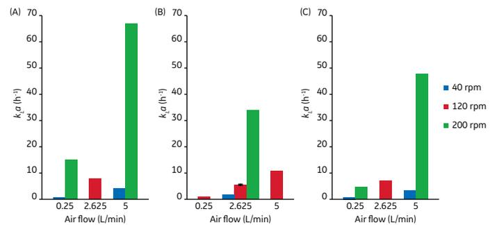
**Fig 10.** Results from the  $k_La$  tests for the 1.0 mm sparger in (A) 15 L, (B) 32.5 L, and (C) 50 L. The DoE center point was replicated in triplicate runs. The error bar corresponds to one standard deviation.
