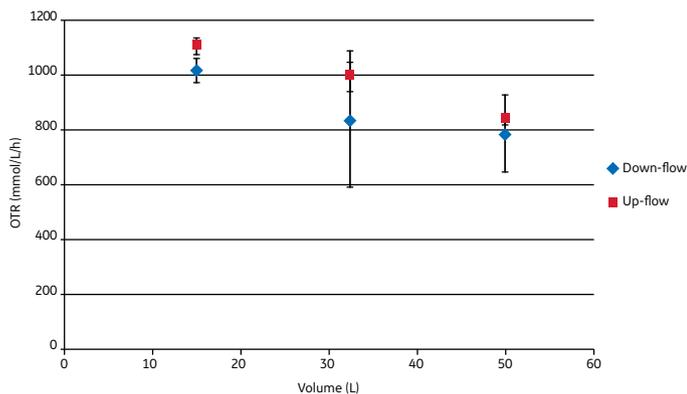
**Fig 15.** Results from  $OTR_{max}$  measurements. Error bars correspond to three standard deviations.
