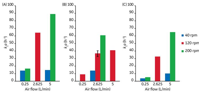
**Fig 7.** Results from the  $k_La$  tests for the 2 µm sparger in (A) 15 L, (B) 32.5 L, and (C) 50 L. The DoE center point was replicated in triplicate runs. The error bar corresponds to one standard deviation.
