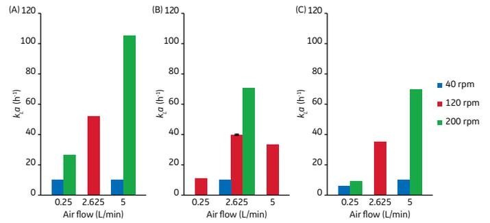
**Fig 8.** Results from the  $k_La$  tests for the 20 µm sparger in (A) 15 L, (B) 32.5 L, and (C) 50 L. The DoE center point was replicated in triplicate runs. The error bar corresponds to one standard deviation.
