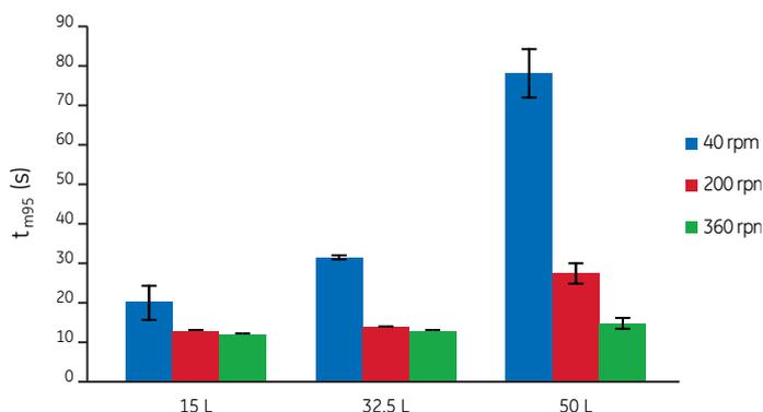
**Fig 4.** Average mixing times ( $t_{m95}$ ) from the probe positions that generated the longest mixing time for all tested volumes and agitation rates. Error bars correspond to one standard deviation.
