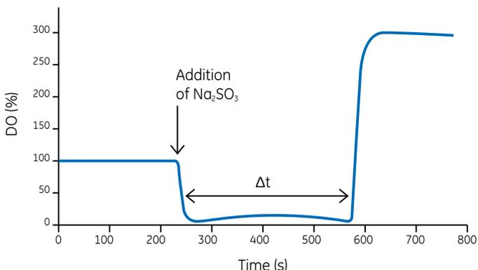
**Fig 3.** DO curve during OTR measurements. The time when DO is below 50% ( $\Delta t$ ) was used for calculating the OTR. The DO reached 300% of air saturation after the reaction was over, as the gas was enriched with 50% oxygen from the time point when  $Na_2SO_3$  was added.
