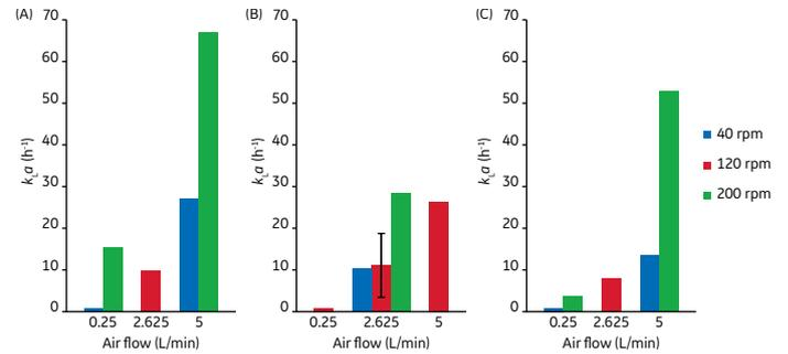
**Fig 9.** Results from the  $k_La$  tests for the 0.5 mm sparger in (A) 15 L, (B) 32.5 L, and (C) 50 L. The DoE center point was replicated in triplicate runs. The error bar corresponds to one standard deviation.
