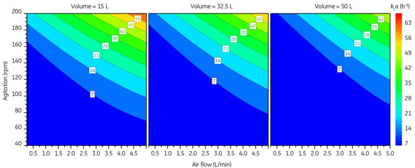
**Fig 14.** 4D response contour plot displaying  $k_La$  obtained with the 1.0 mm sparger pore size at varying air flow, volume, and agitation. The model fit ( $R^2$ ) is 0.98, the model predictability ( $Q^2$ ) is 0.92, and the residual standard deviation (RSD) of the model is  $3.44 \text{ h}^{-1}$ .
