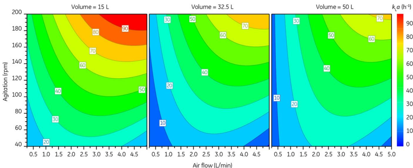
**Fig 12.** 4D response contour plot displaying  $k_L a$  obtained with the 20  $\mu\text{m}$  sparger pore size at varying air flow, volume, and agitation. The model fit ( $R^2$ ) is 0.98, the model predictability ( $Q^2$ ) is 0.93, and the residual standard deviation (RSD) of the model is  $5.28 \text{ h}^{-1}$ .
