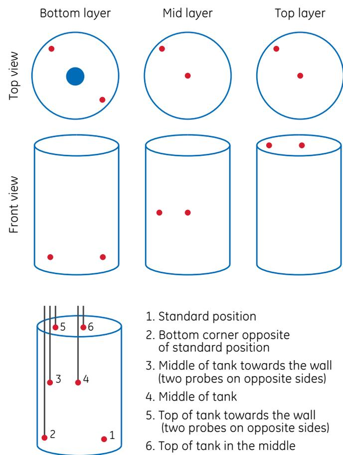
**Fig 2.** The pH probe positions at maximum working volume (50 L). At 32.5 L, probe number 5 and 6 were lowered as much as the water level and probe number 3 was lowered to be positioned in between probes 5/6 and 2. Probe 4 was disconnected. At 15 L, all probes except number 1 and 2 were disconnected. The acid and base were added at the top as close to the center as possible.
