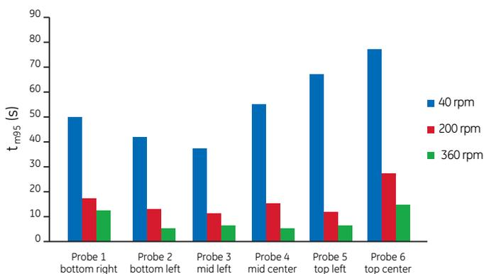
**Fig 5.** Mixing time ( $t_{m95}$ ) for each probe position for maximum working volume (50 L), tested at low, mid-point, and high agitation. Results are averaged values from duplicate runs.
