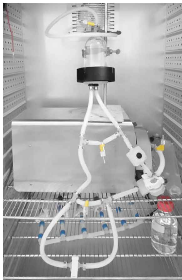
Fig 5. Filling and circulation procedure of ÄKTA ready Low Flow Kit in an incubator. The peristaltic pump is placed behind and connected to the pump tubing. The bottle with the control sample is seen to the right.
