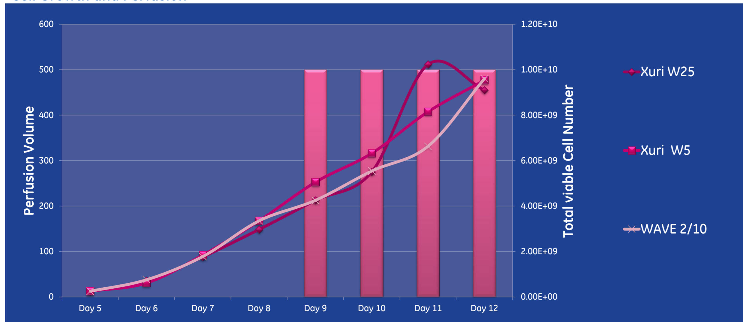
Figure 4. Shows total viable cell number, right hand axis and total perfusion volume, left hand axis, for the redesigned Xuri Cellbag on each platform.
