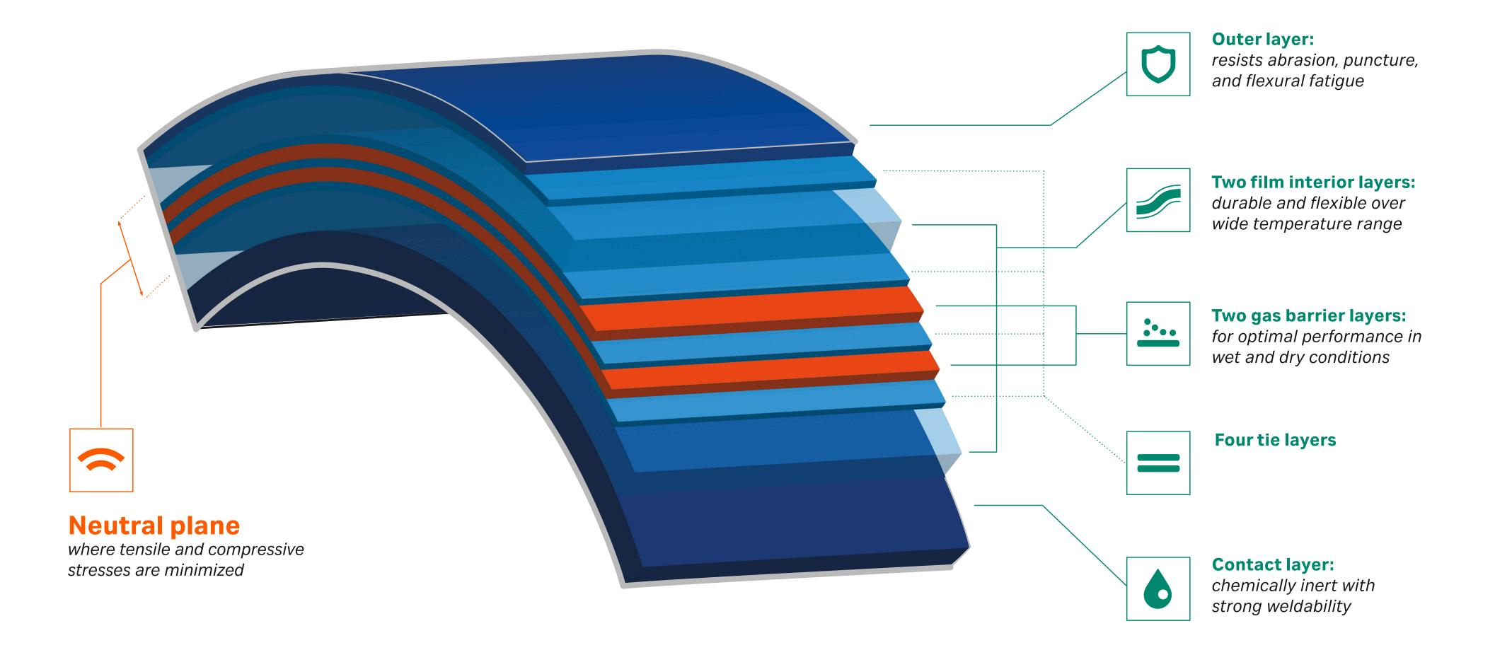
Co-extruded film manufactured in Class 8 cleanroom. Supplied as double ply: contact layer exposed only to Class 5 air (Sealed Air Corp. film design patent).
