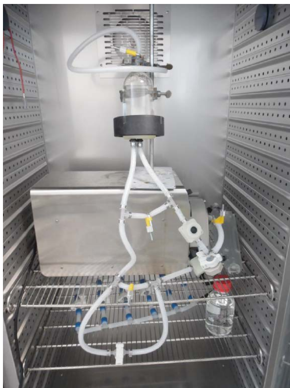
Fig 4. Filling and circulation procedure of ÄKTA ready Low Flow Kit in an incubator. The peristaltic pump is placed behind and connected to the pump tubing. The bottle with the control sample is seen to the right.
