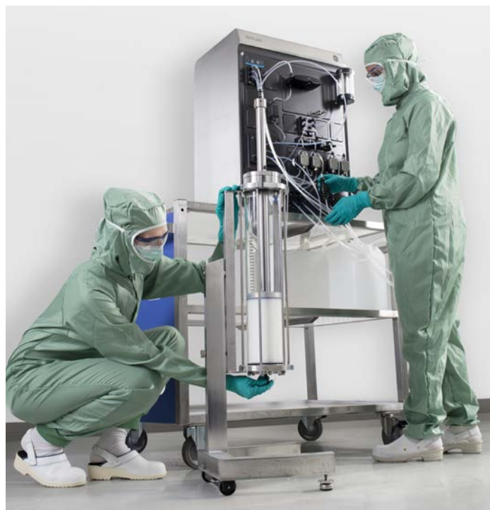
Fig 1. ÄKTA pilot 600 bench-top chromatography system can be used in both GMP ("regulatory" version) and non-GMP ("standard" version) environments.
