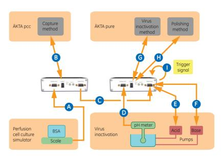
The unit operations in this setup can run three different types of UNICORN methods, *Capture*, *Virus inactivation*, and *Polishing*.
