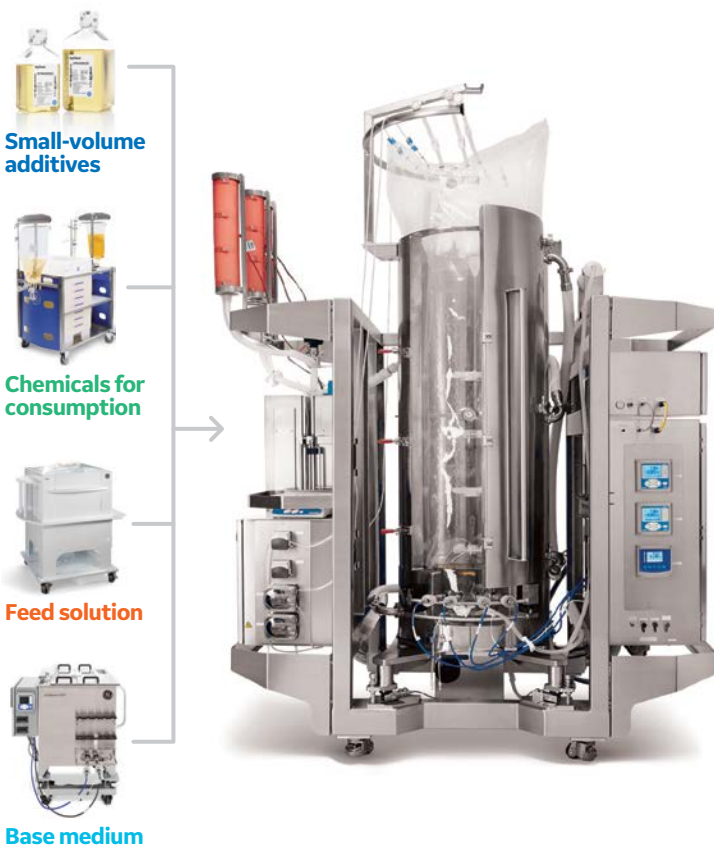
Fig 3. Single-use fermentation medium preparation equipment and supplies.
