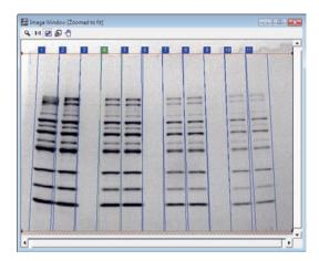
Image elements that are not related to lanes may confuse automatic lane detection. For best results, set an area of interest (*Specifying an area of interest*, *on page 45*) or crop the image (crop image) to exclude the edges of the gel from the image.
