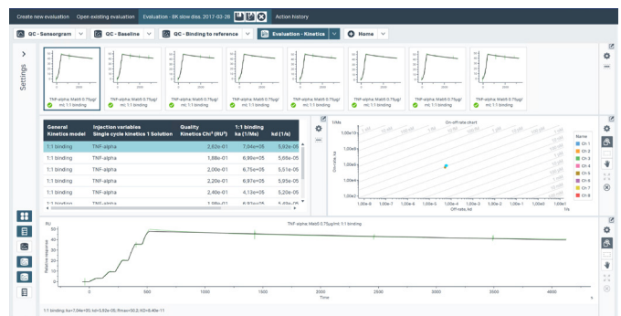
Fig 3. The flat interface of Biacore Insight Evaluation Software provides full overview while offering flexible tools for customized data analysis. The overview allows convenient simultaneous visualization of kinetics and affinity data providing Result table , On-off rate chart , and K d chart .
