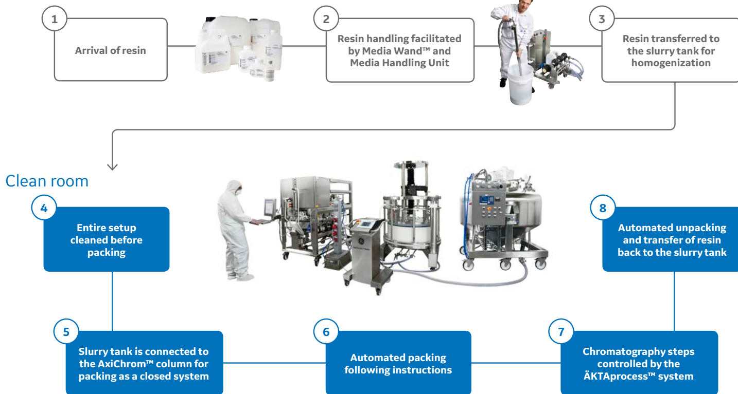
Fig 4. Column packing in a closed system means manual handling of resin and buffers is kept to a minimum. This is achieved by connecting the column, slurry tank and chromatography equipment in a closed system (blue boxes).
