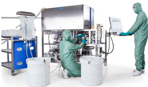
Fig 5. In-line conditioning from HyClone™ buffer stock solutions and WFI reduces manual operations and exposure to contamination
