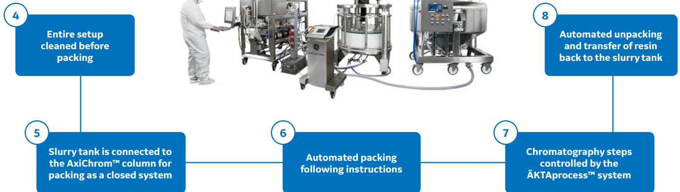
Fig 4. Column packing in a closed system means manual handling of resin and buffers is kept to a minimum. This is achieved by connecting the column, slurry tank and chromatography equipment in a closed system (blue boxes).
