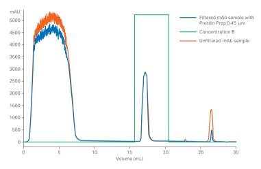
Fig 1. mAb purification on a 1 mL HiTrap™ MabSelect™ PrismA column run on ÄKTA pure™ 25 chromatography system. Detection was performed at A280 nm.
