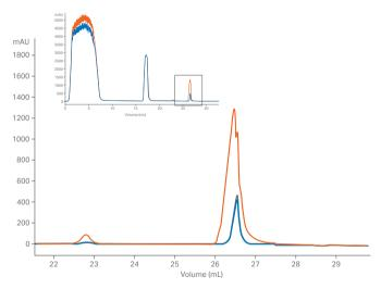
Fig 2. The clean-in-place (CIP) peak after purification of the unfiltered (orange) and filtered (green and blue) mAb samples.
