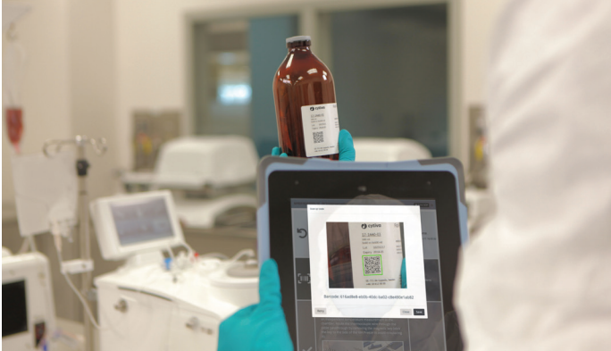
Fig 3. Operators can scan a reagent label to identify lot number and expiration date.
