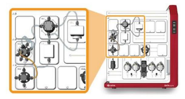
The intermediate peak is directed to the sample loop on the Injection valve before going on to the second column.
