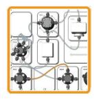
Peak collect tubing between Mixer valve position ReInj and Outlet valve position Out (V9-Os) OR Out 2 (V9-O)
