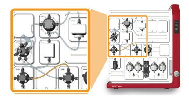
The intermediate peak is directed to the sample loop on the Injection valve before going on to the second column.
