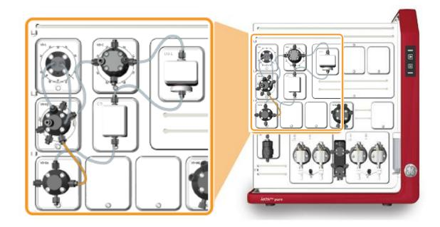
The intermediate peak is directed to the sample loop on the Loop valve before going to second column.
